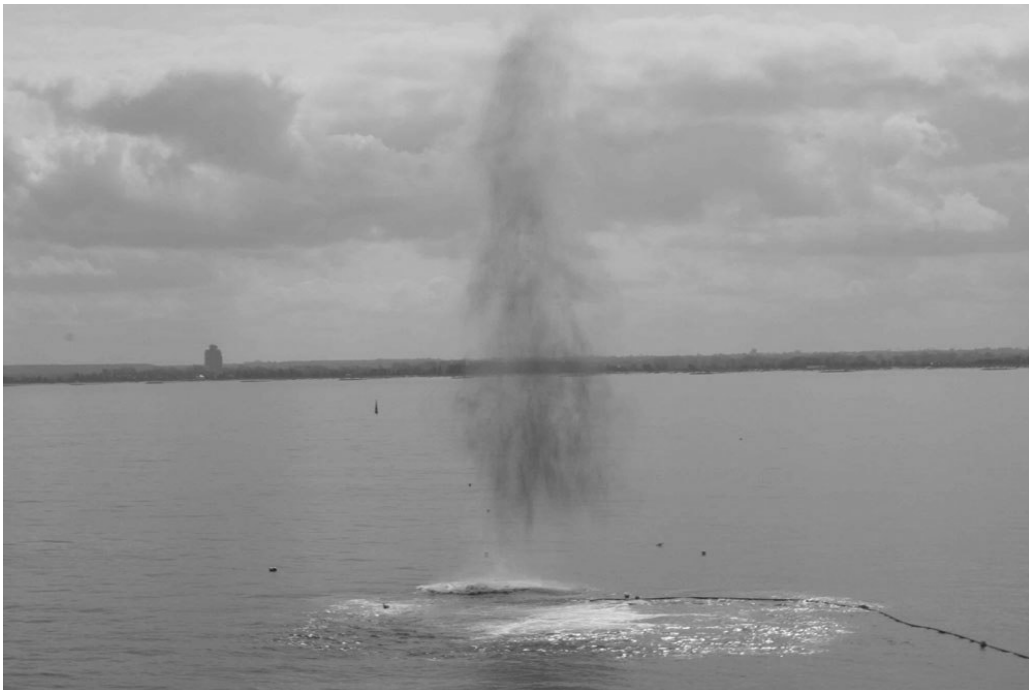
Fig. 1: Test detonation when using a bubble curtain
