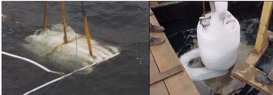
Fig. 2: Ammunition salvage using freezing. Demonstration in the Baltic, © North Sea Divers, Ammersbek, Germany
